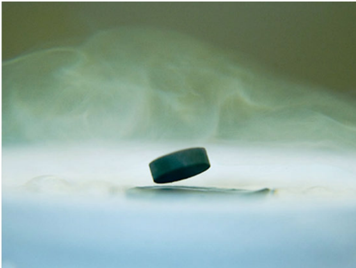
Figure III.3.16: Magnetic levitation . A little magnet will be lifted above a superconductor, because of the Meissner effect, which means that magnetic field lines are expelled from a superconducting region. The aura of magic is caused by the boiling liquid nitrogen needed to cool the high-temperature superconductor. (Source: Michigan State University.)
