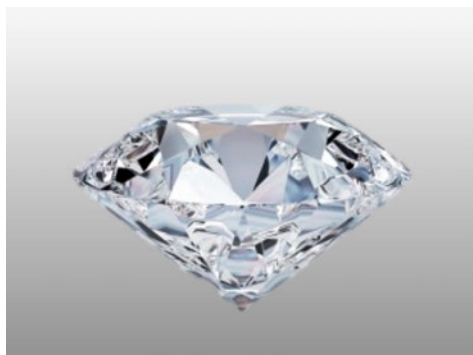
(a) The facets of a diamond are designed to maximize its reflections.
