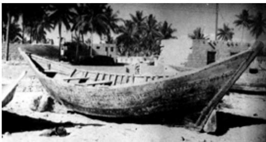
**Figure 4.8** Second photograph of a sewn-plank boat from Zafar, Oman
