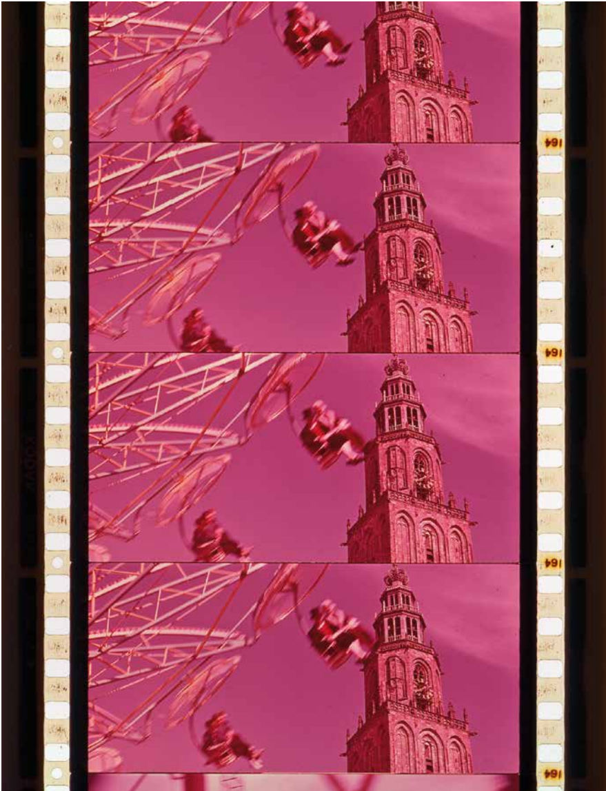
Fig. 8: Example of color fading in a film print of Sky over Holland (John Fernhout, NL, 1967 – courtesy of Eye Filmmuseum).
