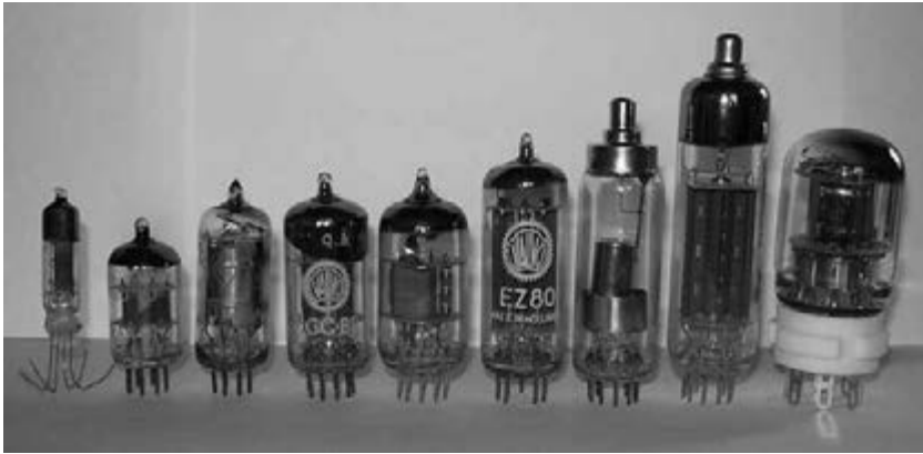
Fig. 12.2: The evolution of diodes as a process of concretization. Photo by Stefan Riepl, licensed under Creative Commons Attribution-Share Alike 2.0 Germany.
