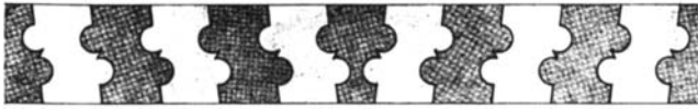
Fig. 7 Detail of joggled string course above lintel of central entrance to Palace of Sitt ʿUnshuq
