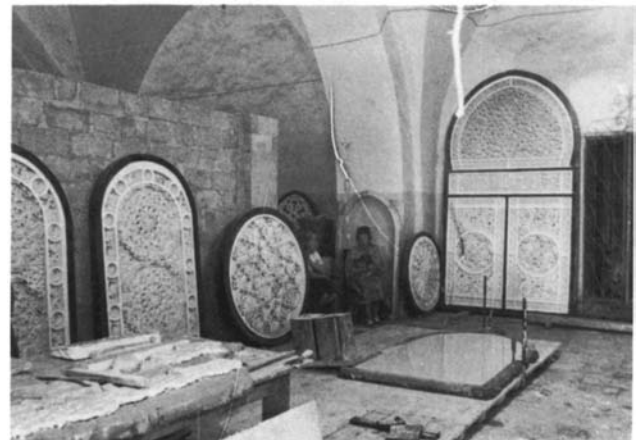
Plate 19 Some finished windows in the workshop, around the qamariyya mould, left to set on the floor
