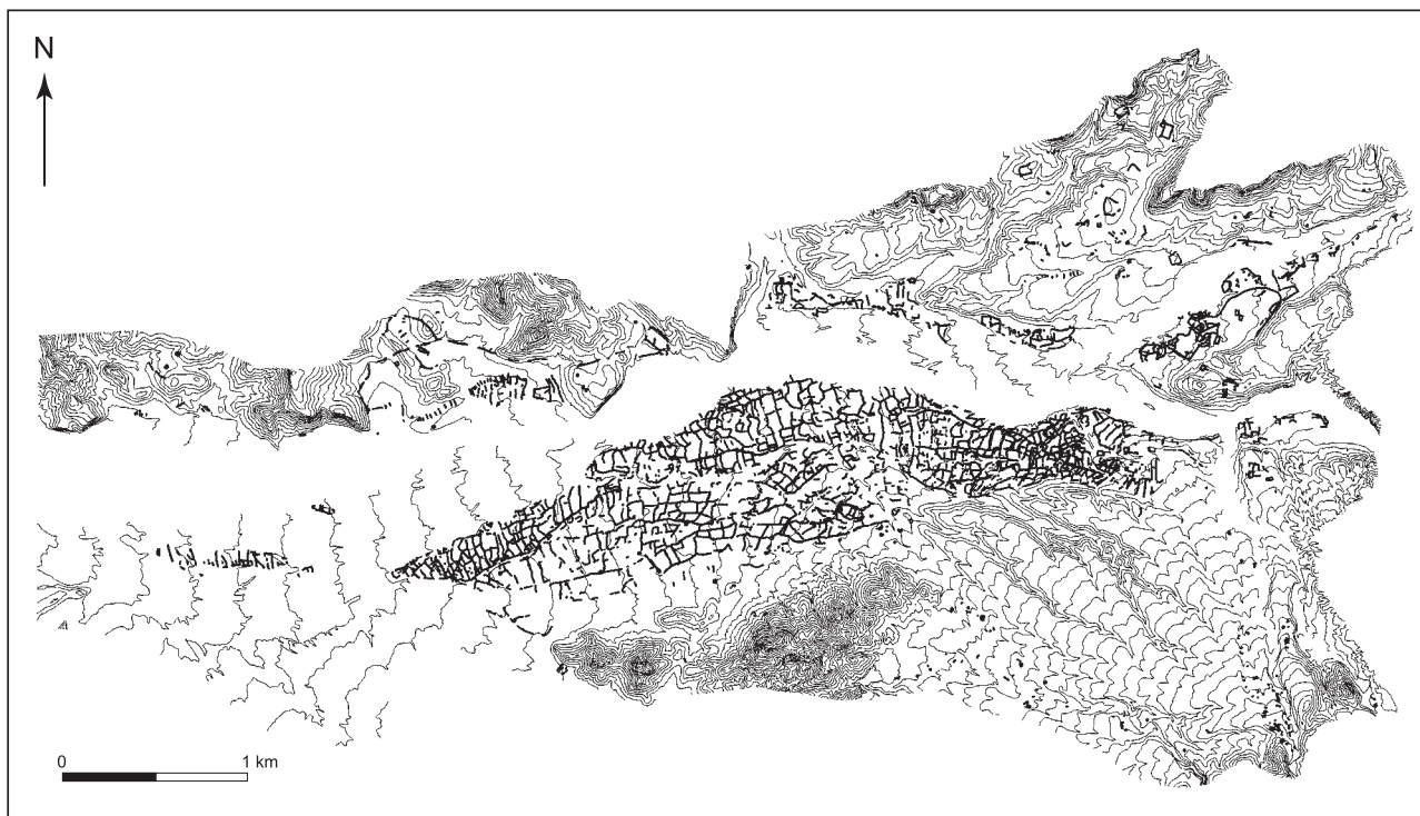
Figure 1.16 The photogrammetric map that formed the primary base map for the survey, limiting the fieldwork until the availability of hand-held GPS technology (for altitudes, see Fig. 1.3).
