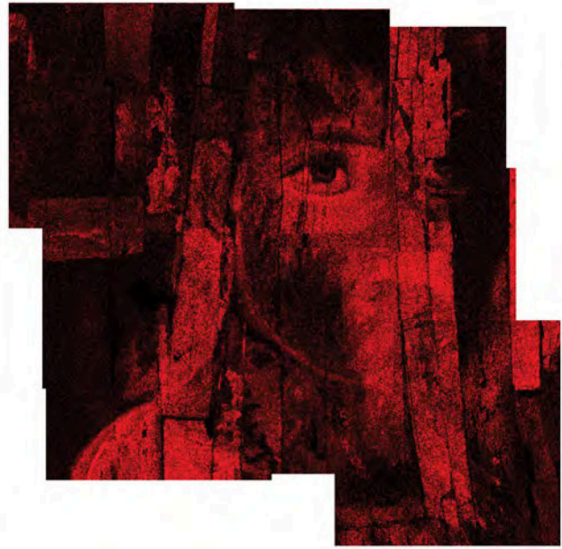
Figure 13.3 Scanning XRF map showing lead on Mummy Portrait of Sarap[i]on. Map obtained on a Horiba XGT-5000 at Georgia Electron Microscopy.
