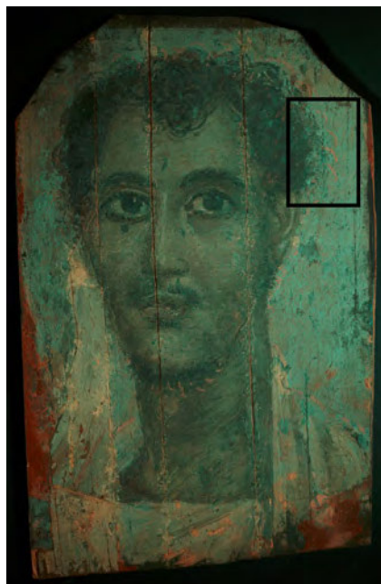
Figure 8.9 VIVL image of fig. 8.1. Camera: Canon EOS D5 Mark III (unmodified); American DJ-brand 64 LED Pro (blue light); Lee no. 16 filter. Image: E. Mayberger and M. Gleeson, Courtesy of the Penn Museum
