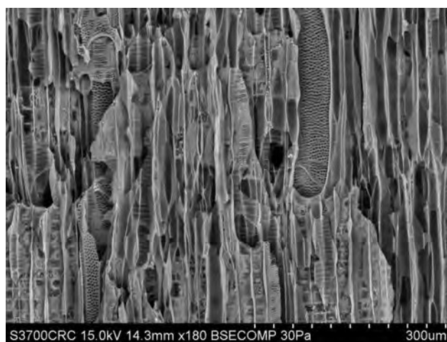
Figure 2.3 SEM image of an RLS of Tilia europaea , lime wood; scale bar is in microns. Image: C. R. Cartwright. © Trustees of the British Museum
