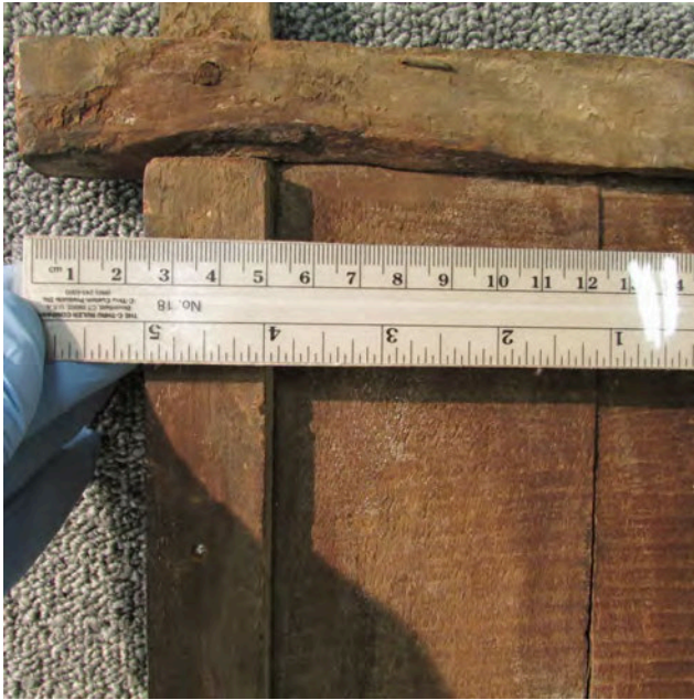
Figure 9.4 Detail of fig. 9.2, showing wane edge and tool marks. Photo: I. Neuman, RISD Museum
