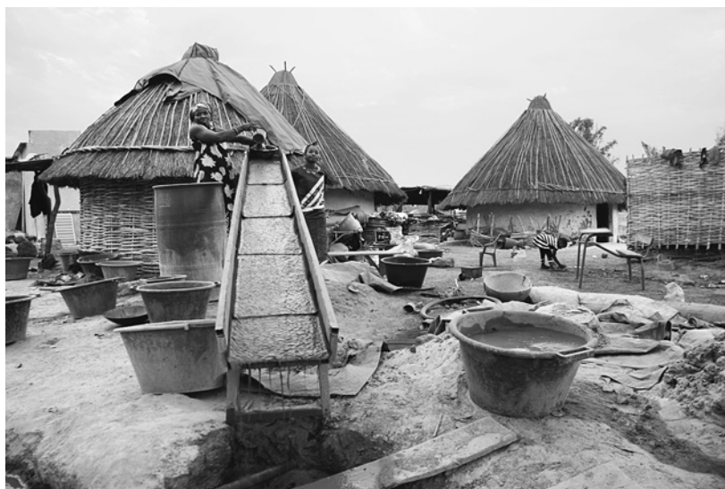
Figure 1.1 Women washing gold by sluice. Tinkoto, Senegal, 2014. Photograph by the author.
