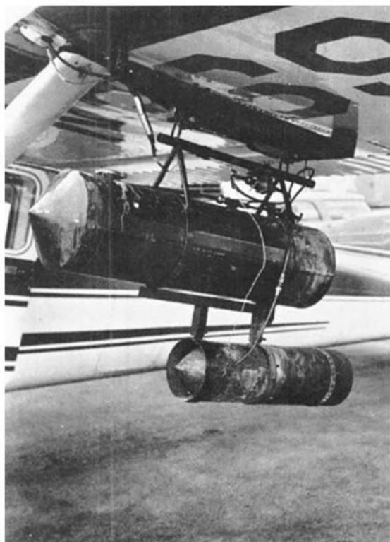
FIGURE 6.3. Project Skyfire airborne silver iodide generator. From Donald M. Fuquay, "Project Skyfire Progress Report, 1958-1960," Intermountain Forest and Range Experiment Station, Forest Service, USDA, Ogden, Utah, 1962.
